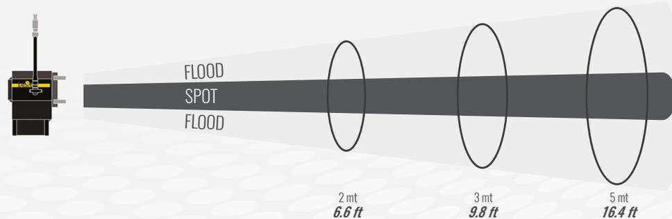
Light beam diameter with Beam Angle (50% of center value)
