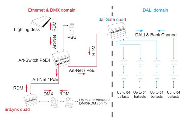
In this example, 3 Artistic Licence products (daliGate quad, artLynx quad and Art-Switch POE4) are used in combination to allow any Art-Net enabled lighting desk to control DALI ballasts alongside DMX fixtures. The Art-Switch POE4 optionally enables the gatways to be powered via the ethernet cable using Power-Over-Ethernet.
