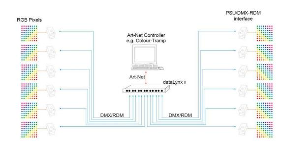
In this example, dataLynx II converts Art-Net from a Colour-Tramp controller into DMX/RDM data. This is fed into intelligent power supplies for use with an LED pixel product.
