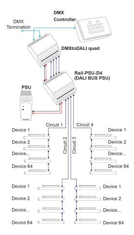
The application diagram shows DMXtoDALI quad being used to its full potential. In this example, a Rail-PSU-D4 is used to provide the DALI bus power supply.
