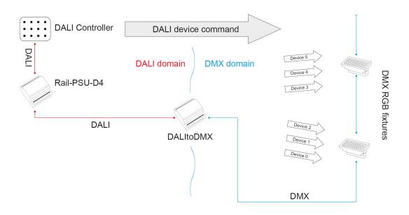
The application diagram shows DALItoDMX used in Device Mode, allowing control over a set of DMX fixtures. A Rail-PSU-D4 is used to provide the DALI bus power supply.
