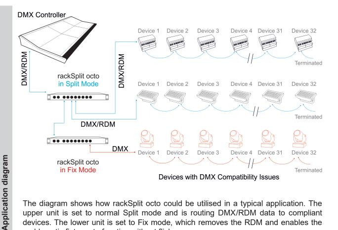
The diagram shows how rackSplit octo could be utilised in a typical application. The upper unit is set to normal Split mode and is routing DMX/RDM data to compliant devices. The lower unit is set to Fix mode, which removes the RDM and enables the problematic fixtures to function without flicker.
