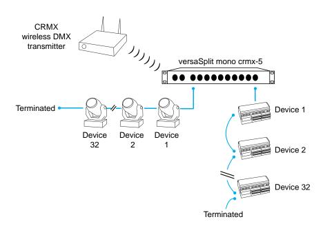
In this example, the maximum number of DMX devices are driven on outputs 1 and 10.
