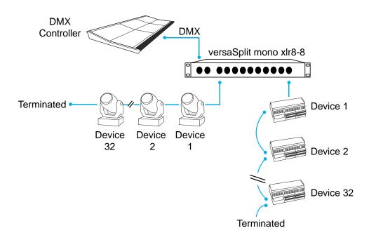
In this example, the maximum number of DMX devices are driven on outputs 1 and 10.
