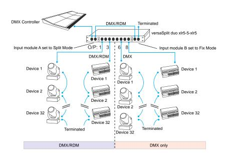
In this example, versaSplit duo xlr5-5-xlr5 is used simultaneously as a DMX splitter and fixer. Input module A is switched to Split mode, while input module B is set to Fix mode. Outputs 1 and 3 are switched to 'A', while outputs 6 and 8 are switched to 'B'. The devices on outputs 6 and 8 see only DMX data, which can be useful in resolving flickering issues arising from non-compatibility with RDM.
