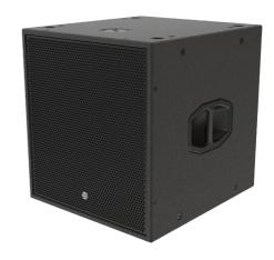
The S-18 requires an active crossover to function correctly – although the choice of filter points is very wide, allowing the user to tailor the response to exactly what is required. Cardioid DSP program settings are also available to create arrays with significant rejection to the rear of the subwoofers, by stacking three enclosures in a block (two facing forwards, one facing backwards).
