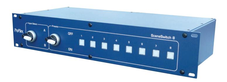
The ProPlex SceneSwitch 8 is an 8-channel DMX A/B switcher with built-in 8-scene playback. Perform rapid switching between two DMX sources, e.g. two lighting consoles or between the main console and a backup. Scene playback captures data on all eight DMX lines and, if a console fails, allows instant recall of eight pre-recorded scenes. DMX source and backup functions are selected with a rugged toggle switch to avoid accidental switching.
