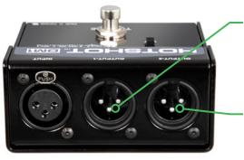
**OUTPUT-A** connects the direct mic output to the main snake system. All XLRs are wired pin-2 hot (AES standard) and isolated from the enclosure.
