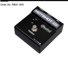
The Radial Hot Shot DM-1 is a combination microphone signal splitter and mute switch that allows the vocalist to depress a footswitch to mute his mic and redirect the signal to the monitoring system and/or intercom. This 100% passive floor-box is equipped with XLR mic input, momentary footswitch, direct and switched XLR outputs.
