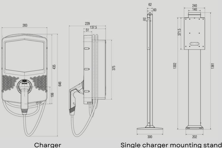
The Chargers are equipped with a type 2 lead and plug. A type 2 charging cable is the European-standard plug type used by every new electric car.
