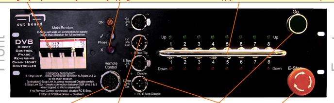
Remote operation of the DV8 is available using the optional RC8 remote control handset, which provides Up/Down switches for motor direction, GO and E-Stop. The RC8 handset is connected to the DV8 via a detachable multicore cable. Two DV8's can be run from one RC16 sixteen-channel handset via an RC Handset Splitter. Programmable control systems such as the IBEX PHC+ can also connect to this Remote Control socket to automate the DV8.
