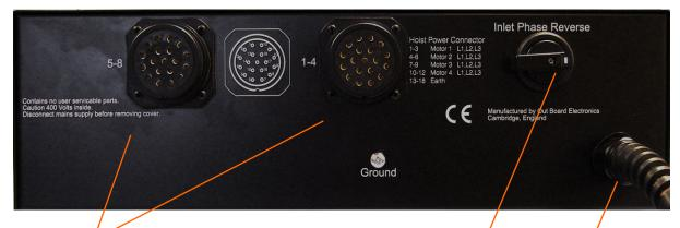
Connections to hoists are arranged on two female 19-way Socapex connectors, in groups of four channels of Up/Down switched 3-phase power and earth on each.
