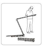
Set frame to desired height then extend legs accordingly and fasten with black knob
