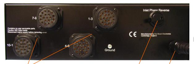
Connections to hoists are arranged on four female 19-way Socapex connectors, in groups of three channels of Up/Down control and 3-phase power/earth on each.
