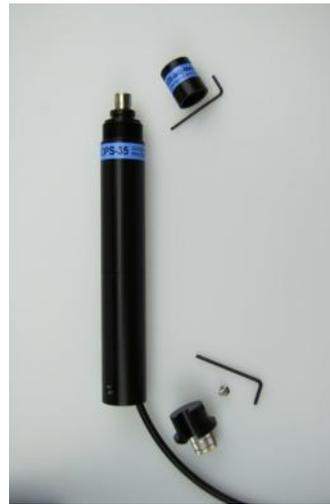
Lift off the adjustment tool and insert the adapter and mic in the OPS35 body. The microphone is installed in the correct position now.
