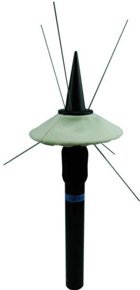
The spikes are securely installed when the bottom holder, the umbrella and weather tip are screwed together (top right picture). There is no need to add glue or epoxy. The cranked ends cannot travel out of the install position even under extreme weather conditions.
