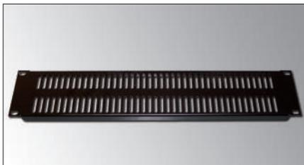
Specifically designed to give extra ventilation in the racks. They are manufactured in 20/10 aluminium plate finished in smooth, black dust, epoxy and have a 90° fold, top and bottom, to give better rigidity.
