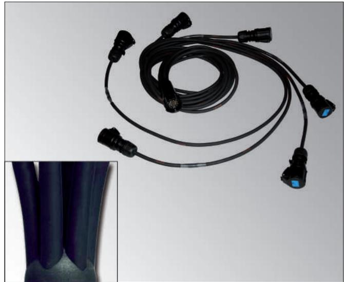
Cord splitter manufactured with 2.5 mm<sup>2</sup> H07 RN-F rubber cable overall length 1 meter, (any length can be supplied too), featuring bare ends or wired with any 16-32A / 100-240Vac sockets or plugs.
