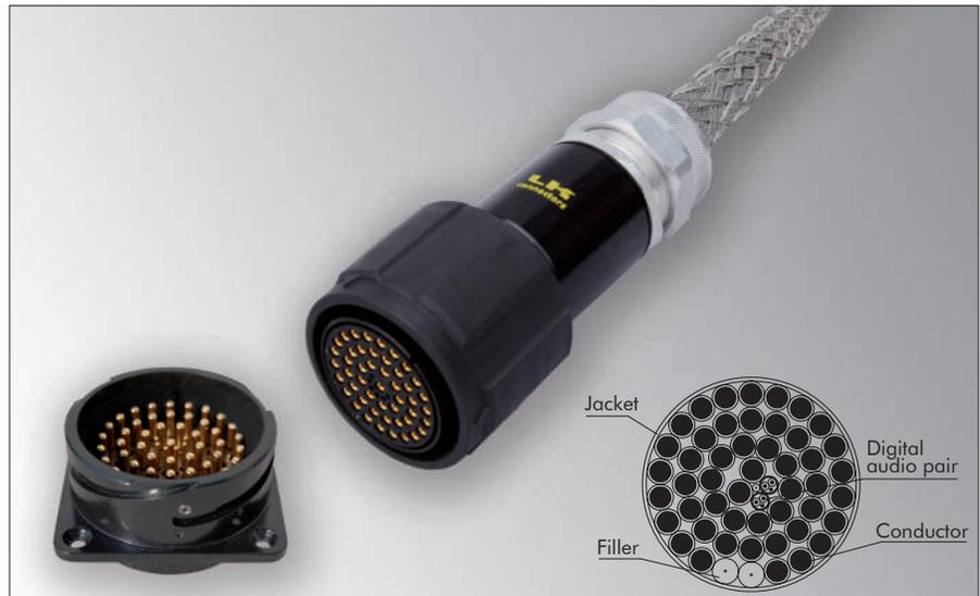
The **LKA 48/6** connector was designed to connect speaker clusters using as few cables as possible. It can carry up to 18 speaker and 2 AES/EBU channels with the **eurocable 36N40AD2** cable or up to 48 speaker and 2 AES/EBU channels with the **eurocable 48N40AD2** cable.
