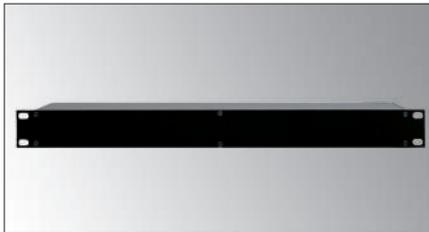
The front and the rear panel are manufactured in 30/10 black finished aluminium plate; they are available in 1, 2 and 3 rack units consisting of a "U" shaped base and top lid. They can be supplied customized with pre-punched and laser labelled holes on the front and rear upon request.
