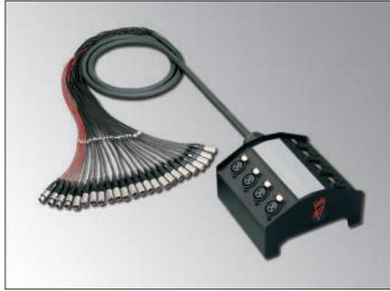
The SBF range features SSA cable (individually shielded multi-pair **eurocable**) hard wired to the XLRs into the box and a XLRs fan out on the other end. The individual pairs are protected by Techflex to maintain ultimate flexibility. Use of coloured Techflex allows the easy identification of fan channels.
