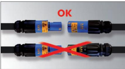
The Power Link connector series has permanent integral keys which prevent the accidental connection of dissimilar types (e.g. Earth and line 1).
