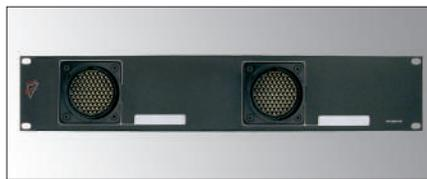
ADF 2RU panels use the capability of the multi-pin LK range to connect from 8 up to 64 audio lines using only one cable. The 26 pin ribbon cable connectors allow XLR connections. They can be used for FOH, Monitor, REC, AUX or other connections, as well as Sub-snake boxes.
