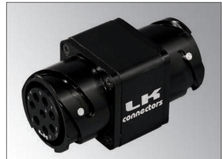
**LKA 16** (crimp pins) and **LKI 16** (solder pins) connectors are based on standard LKS Socapex style connectors but have been adapted to use only 16 pins, following indications from the largest rental companies. The standard Socapex style LKS 19 pin connector is also available, as utilized by D&B. Rubber locking ring available on both bayonet style and screw coupling connectors.
