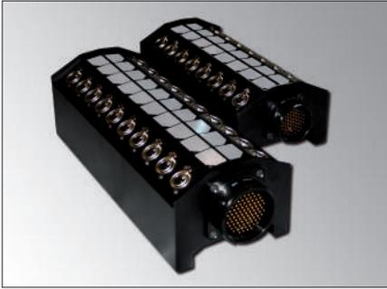
The compact design and its raised bottom, simplify the use in narrow space allowing the cables to be gathered beneath it. The SB box mounts a LK multipin panel connector for an easy cable disconnection.
