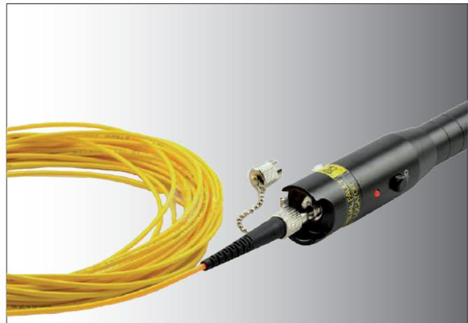
Pen Shape **Visual Fault Locator** is a compact but powerful fiber optical cable test tool, with an output power up to 10mW, which can be used to locate sharp bends & breaks in jacketed or bare fiber at more than 10km. It can also be applied to identify the connectors in patch panels and identify the fibers during splicing operation. The choice of a continuous wave output mode for steady fault illumination or a flashing output mode makes easier fault location possible.
