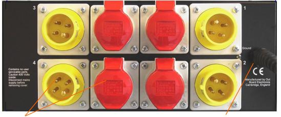
Connections to hoists are arranged on individual Yellow male 4-pin C-Forms for Up/Down control and Red female 4-pin C-Forms with switched 3-phase power/earth on each.
