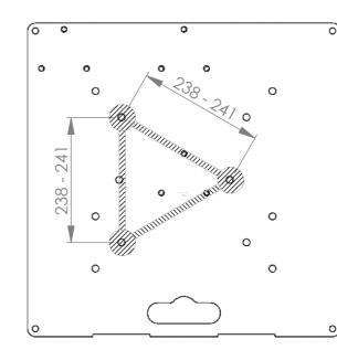
TANK TRAP BASE USED AS TRUSS MOUNTING PLATE
