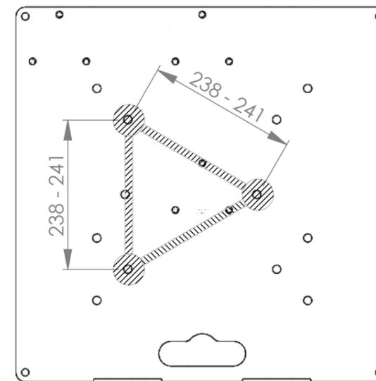
TANK TRAP BASE USED AS TRUSS MOUNTING PLATE
