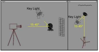
the camera. From a side view, raise the Key Light above the camera, so that it hits your subject from about 15 to 45 degrees higher than the camera angle.
