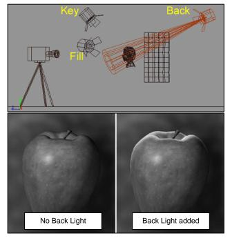
That's it. Three-Point Lighting can be a simple starting-point for lighting just about any subject. In a more complex scene, there are other types of lights used as well: Practical Lights, Bounce Lights, Kickers, and Specular Lights, which serve other visual functions.
