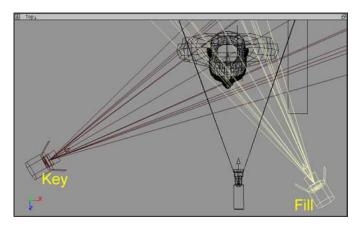
the subject's height, but should be lower than the Key. At most, Fill Lights can be about half as bright as your Key (a Key-to-Fill ratio of 2:1). For more shadowy environments, use only 1/8<sup>th</sup> the Key's brightness (a Key-to-Fill ratio of 8:1). If multiple Fills overlap, their sum still shouldn't compete with the Key. Shadows from a Fill Light shall be very, very Soft.
