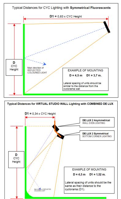
in the direction of the PRESENTERS. For this reason it is strongly recommended to utilise ASYMMETRICAL LIGHTING FIXTURES purposely designed for this application.
