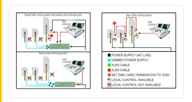
Dimming fluorescent lights is necessary to balance the light level of the different sections of the studio. The use of very high frequency ballasts guarantees color temperature stability, flicker-free and noiseless operation.
