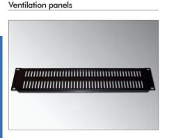
**S**pecifically designed to cover empty units, thereby giving extra ventilation in the racks. They are manufactured in 20/10 aluminium plate with a 90° fold, top and bottom, to give better rigidity.
