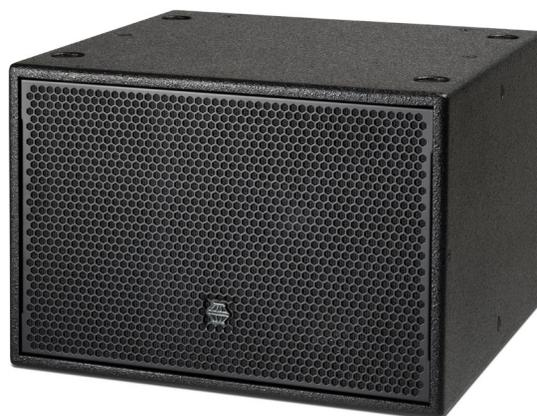
The i-R12 is a compact reflex loaded subwoofer designed to extend the bandwidth and increase the headroom of EMS series mid-high and full range loudspeaker models. It consists of a 12" (305mm) neodymium low frequency driver in reflex loaded enclosure designed to provide smooth LF rolloff and extended bass response.
