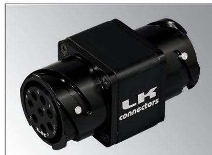
**LKA 16** (crimp pins) and **LKI 16** (solder pins) connectors are based on standard LKS Socapex style connectors but have been adapted to use only 16 pins, following indications from the largest rental companies. The standard Socapex style LKS 19 pin connector is also available, as utilized by D&B. Rubber locking ring available on both bayonet style and screw coupling connectors.
