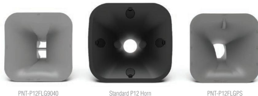
The dispersion characteristics of the P12 can be changed in seconds through the addition of optional magnetic flanges. The standard cabinet uses a 60° x 60° horn with additional 90° x 40° and Asymmetrical (PS Type) 60° - 100° x 40° also available.
