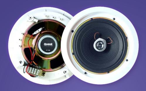
The Quest Q-Tech series QTC1080 ceiling speaker is a 5 taping 15 watt 100/70V line 2-way speaker that is optimised for wide dispersion high intelligibility vocal coverage in commercial environments.
