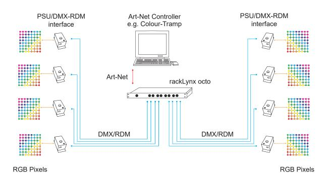
In this example, rackLynx octo converts Art-Net from a Colour-Tramp controller into DMX/RDM data. This is fed into intelligent power supplies for use with an LED pixel product.
